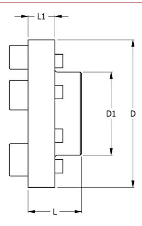
D = 160 D1 = 95 L = 60 L1 = 28 Max bore = 58 Torque (N m) = 560
